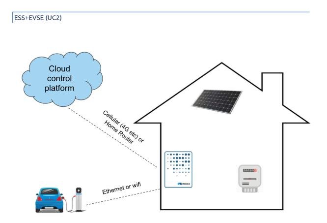
*Figure 5: Control architecture for battery and electric vehicle charger*
