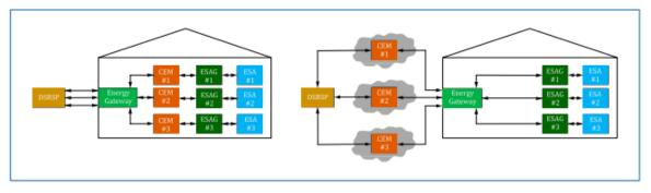
Figure B.2 – Multiple DSRSPs each controlling their own set of ESAs in a premises
