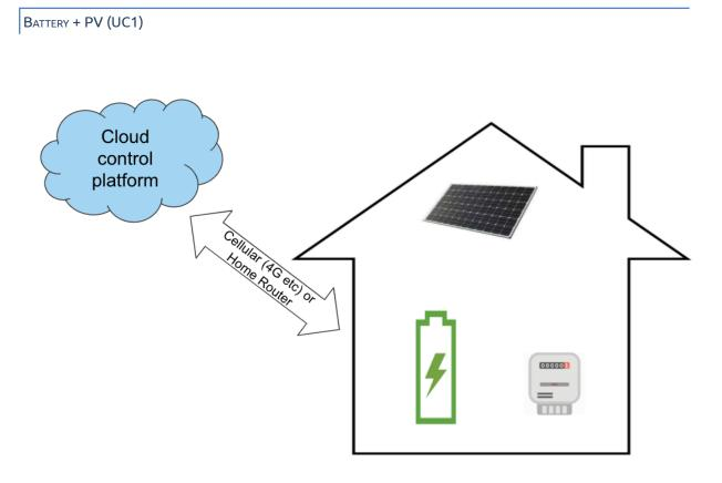
Figure 4: Control architecture for remote ESS control
