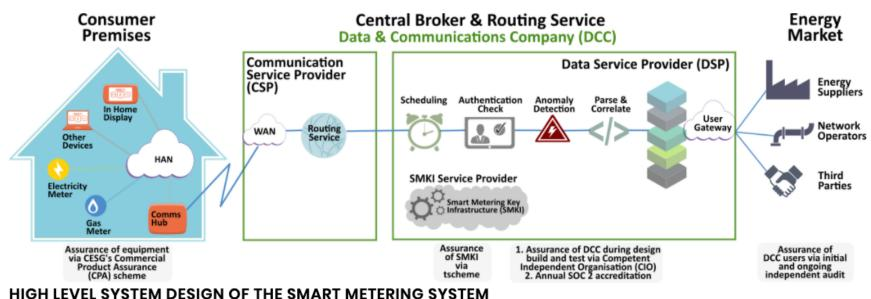
figure 10: DCC communication system schematic from ref;
