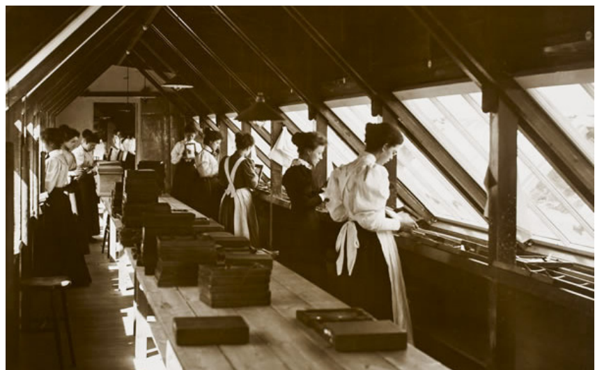
Printing photographs by sunlight at the Kodak factory, Harrow, 1890s © The British Library Board
