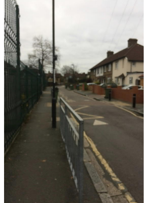
Haimo Road, outside the main school entrance, looking south-east. Note the 'keep clears' and the uncontrolled crossing on the raised table
