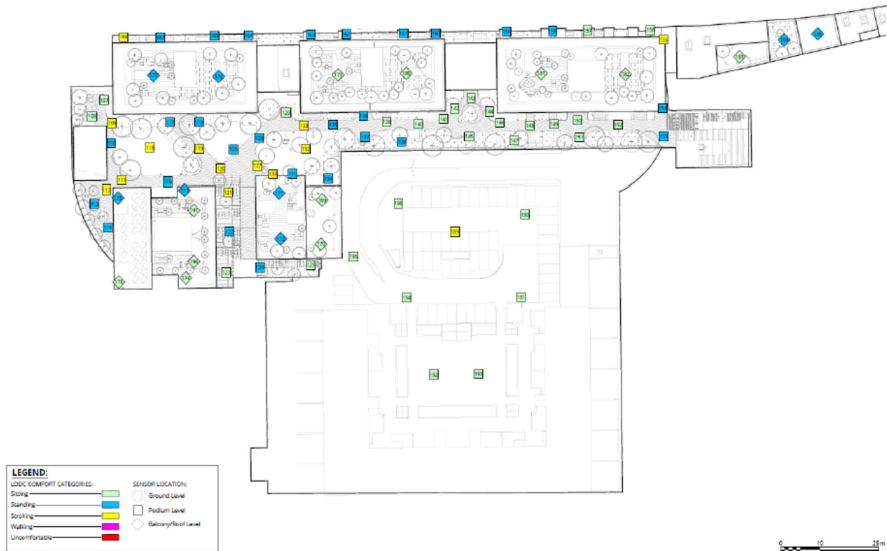
Figure 10.14 Configuration 3: Pedestrian Comfort for the Proposed Development with Existing Surrounding Buildings, Landscaping Scheme, and Wind Mitigation Measures – Upper levels, Windiest Season
