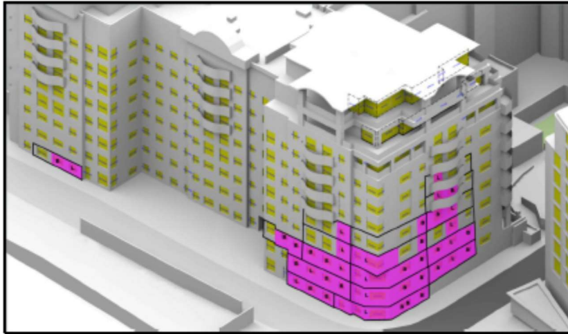
Figure 30: Location of rooms in Warren and Atwood House that would experience major reductions in daylight (shown in magenta)
