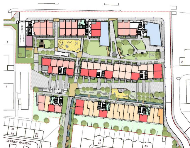
Figure 2: Proposed ground floor plan - Plot A (taken from 10046-A-DRG-Z0-G100-2000-PL-RS Rev E)
