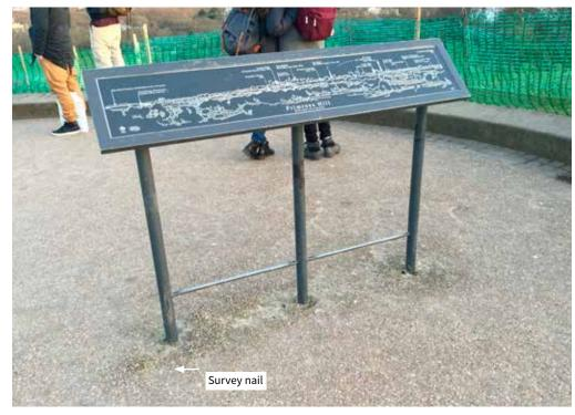
The survey nail near the new orientation panel (right) is about 10.5m away from the real assessment point in the new turf (left).
